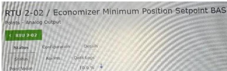
8. Setpoint for position of outdoor air dampers during economizer operation
